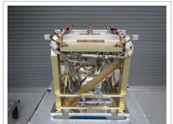
A green propellant propulsion subsystem was recently delivered to Ball Aerospace for integration into the Green Propellant Infusion Mission spacecraft. The subsystem will be one of three experimental payloads on the spacecraft. Photo courtesy of Ball Aerospace
