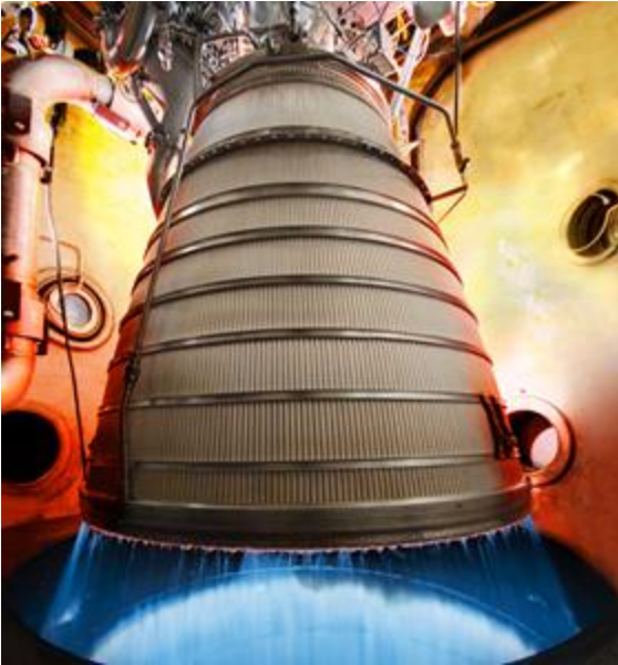
Aerojet Rocketdyne's RL10 engine undergoes testing in West Palm Beach, Florida. The RL10 is the upper-stage engine for NASA's SLS rocket that will return humans to the Moon.
