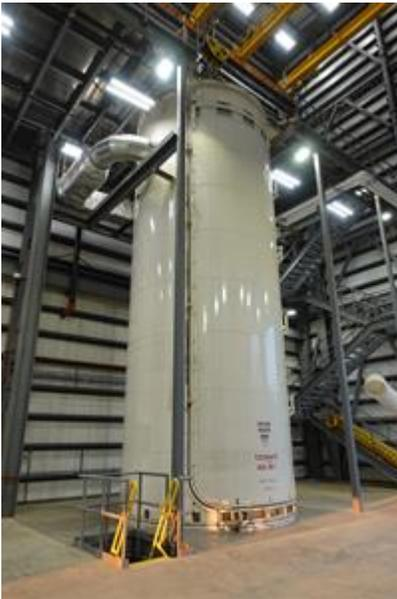
Aerojet Rocketdyne's vacuum chamber casting bell will support production of large solid rocket motors in Camden, Arkansas
