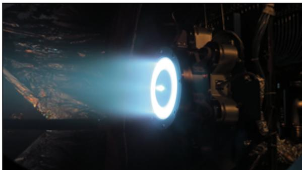
Aerojet Rocketdyne's Advanced Electric Propulsion System thruster demonstrates full power operation at the Jet Propulsion Laboratory in Pasadena, California
