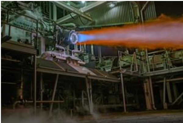
An Aerojet Rocketdyne RL10C-X prototype engine, which includes 3-D printed core components, undergoes hot-fire testing at Aerojet Rocketdyne's facility in West Palm Beach, Florida
