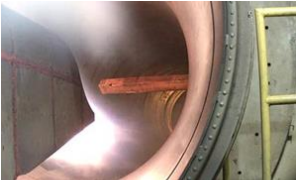
Aerojet Rocketdyne's new dual-mode ramjet/scramjet undergoes testing in the 8-foot high temperature tunnel at NASA's Langley Research Center in Hampton, Virginia
