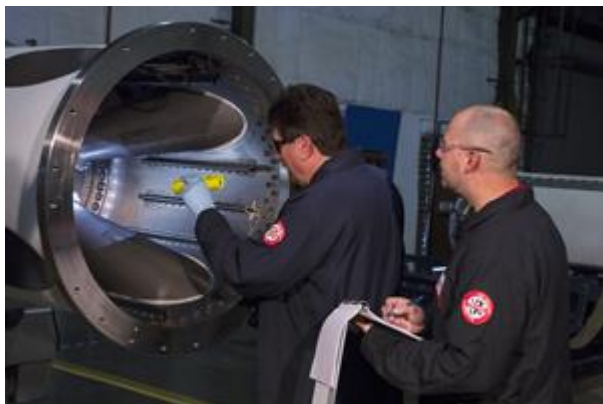
Aerojet Rocketdyne technicians inspect the Jettison Motor for the Lockheed Martin-built Orion spacecraft's Launch Abort System (LAS) at its facility in Sacramento, Calif.
