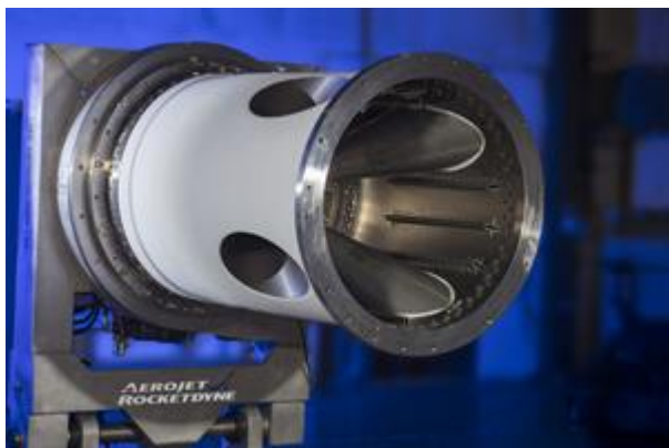
The Jettison Motor built by Aerojet Rocketdyne for the Lockheed Martin-built Orion spacecraft's Launch Abort System (LAS) that will be tested during the Ascent Abort Test (AA-2) next year.
